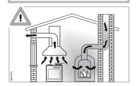
Great care should be taken when using the cooker hood at the same time and in the same room or area of the house as another heating appliance which depends on the air in the room. Such appliances include gas, oil, wood or coal-fired boilers and heaters, continuous flow or other water heaters, gas hobs, cookers or ovens which draw air in from the room and duct exhaust gases out through a chimney or extraction ducting.
